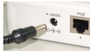
Fig. 8. Connect the power adapter to the HotSpot Gateway.
