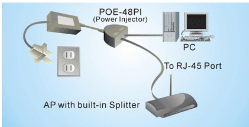
e.g. above shows a LAN cable, with data, coming from a PC. The injector takes in the data cable and inserts the power into the ongoing LAN cable going to the wireless AP. The AP has a built in 'splitter' which extracts the power from the LAN cable and passes it internally onto the built in power circuits. This is an AP with built in PoE capability.
