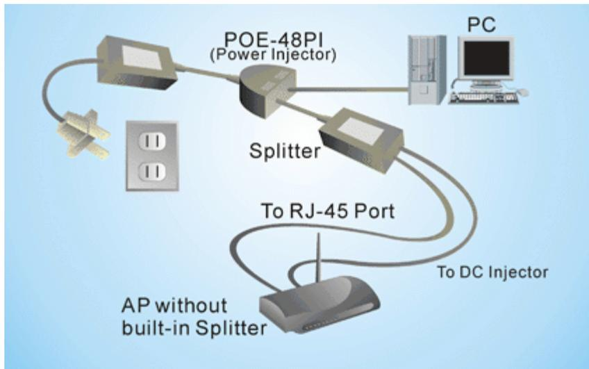
So, in above, the splitter is connected to the LAN cable from the injector. Then, from the splitter, there are two cables going to the AP: One is a short data only LAN cable, the other is a short DC power lead. Generally the splitter does more than just split out the 48V from the LAN cable; it normally performs a second function of 'dropping' the 48V to the native power voltage required by the device e.g. 12 or 5V.
