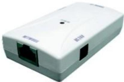
This is a fully 802.3af compliant 48V PoE injector using the Alternative B system (uses the Base 10/100 LAN unused wires). In operation it's very similar to the NET-POEINJECT48 product (detailed above) in that it delivers the 48V DC power using the 'spare' wires however, unlike the POEINJECT48 product, it's fully compliant to the 802.3af standard and as such correctly applies the pre-power delivery tests to ensure that the PD (Powered Device) is capable of accepting 48V power over the LAN port.
