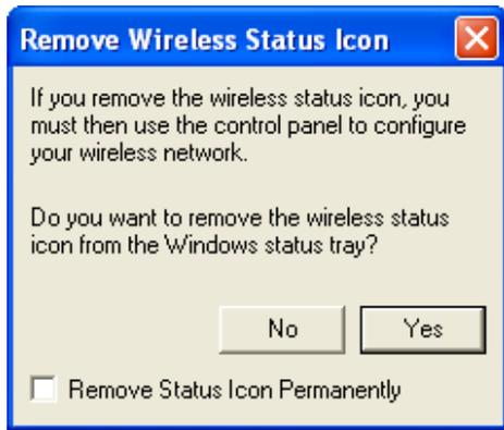
You can also set the system tray radio icon to disappear permanently by placing a check in the box **Remove Status Icon Permanently** as shown above. When the computer is restarted, the system tray radio icon will reappear unless the **Remove Status Icon Permanently** box was checked.
