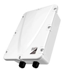
**ENH210** Wireless Outdoor Enterprise Client Bridge features 14dBi high gain antenna dual polarization with high output power and high sensitivity can extend the transmission range to deliver a stable wireless connection. ENH210 integrates 4 operation modes: Access Point, Client Bridge, Client Router and WDS.
