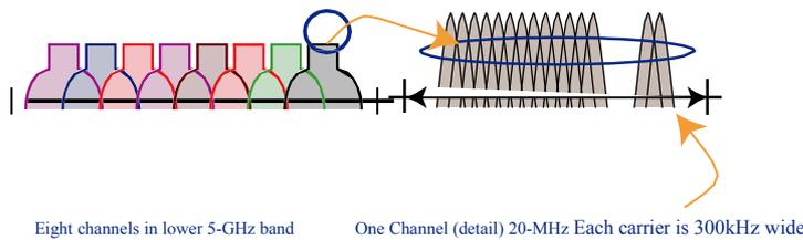
5GHz 54meg (the old 11a standard) or 11n or 11ac wifi all use OFDM to define a number of non-overlapping channels and each of these channels is divided into multiple subcarriers. By comparison the 2.4GHz ISM band used for wifi only has 3 non-overlapping channels.
