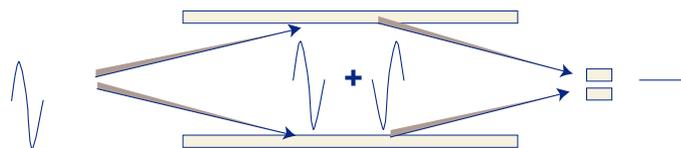
OFDM (orthogonal frequency division multiplexing) modulation is the answer. OFDM is used by 5GHz devices (and also 11g, 2.4GHz devices) and has been growing in usage due to its ability to overcome many of the signalling shortcomings of earlier WiFi technology like multi-path fades.
