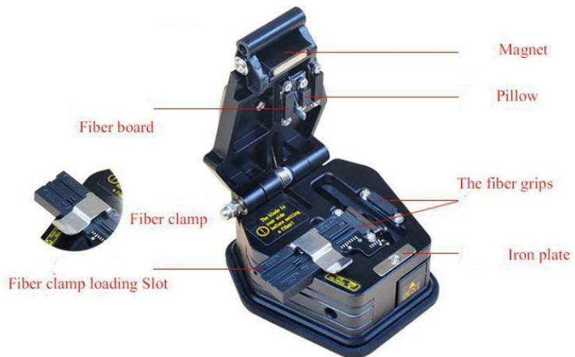
1. Trim the fibre's sleeve and coating to appropriate lengths depending on the connection you are making. Leave at least 20mm of excess fibre projecting beyond the cleave point. This will ensure that the fibre is correctly clamped and that you can safely recover the piece of waste fibre.
