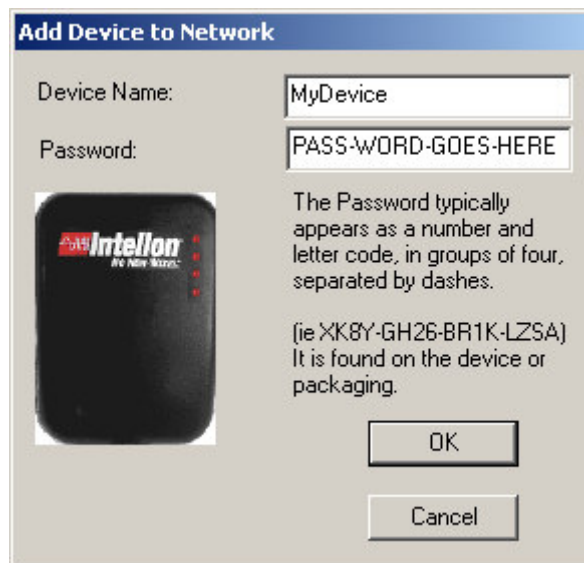
Figure 1-9 : Adding Device To Network
