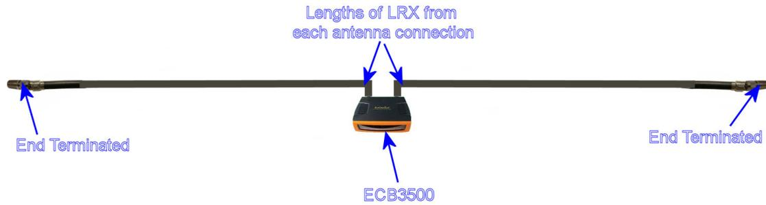
This allows you to run a double length of LCX cable from the same AP without requiring a signal booster or such. Please note if you want to run two lengths this way then the AP must be able to run true, full diversity i.e. it can transmit and receive from both antenna connections.
