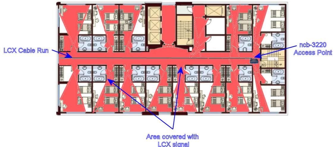
With LCX cable running down the ceiling of the corridor then coverage is much more complete. Basically any point that can 'see' the cable can receive a good signal.
