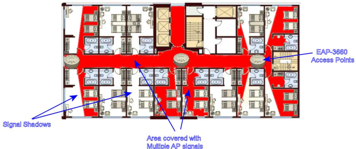
Because of shadows caused by the walls of the rooms and corridor then coverage in those rooms out of line of site of an AP can be very poor. The red areas show where the signal is very strong but note the shadows where signal is not reaching.
