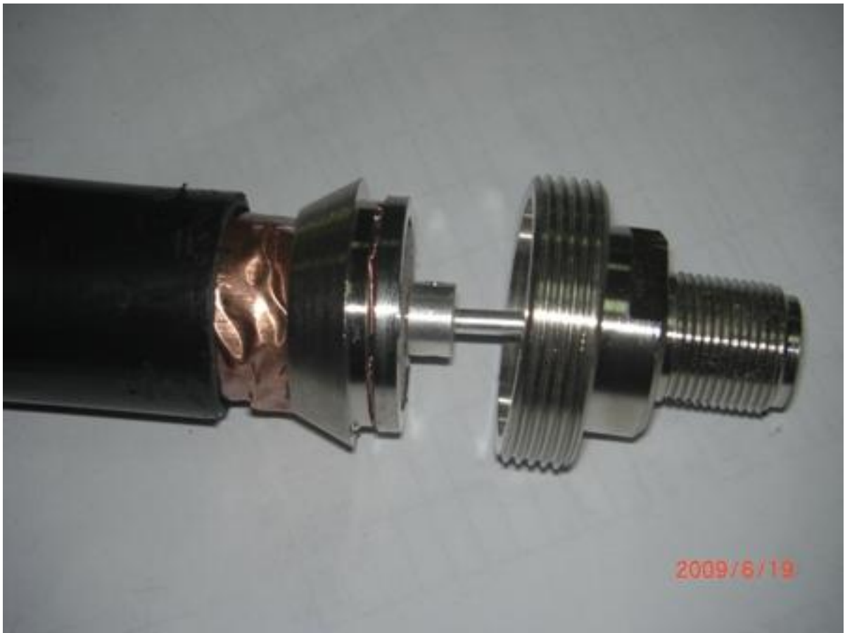
Put front body onto connector inner pin
