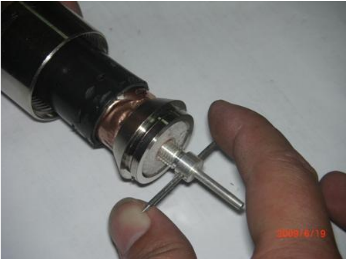
Screw the pin from connector into cable inner conductor
