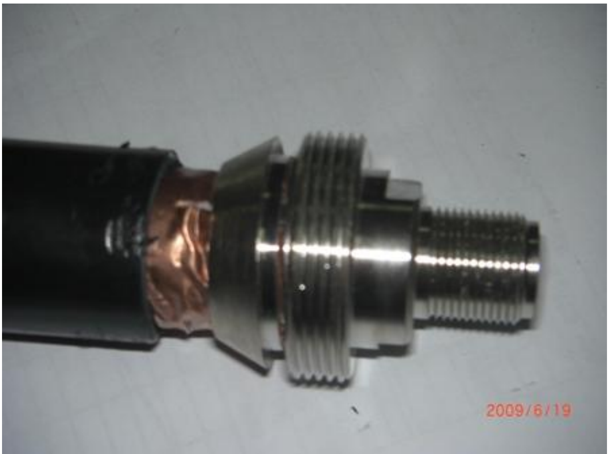
Screw front body up tight to the end of the cable
