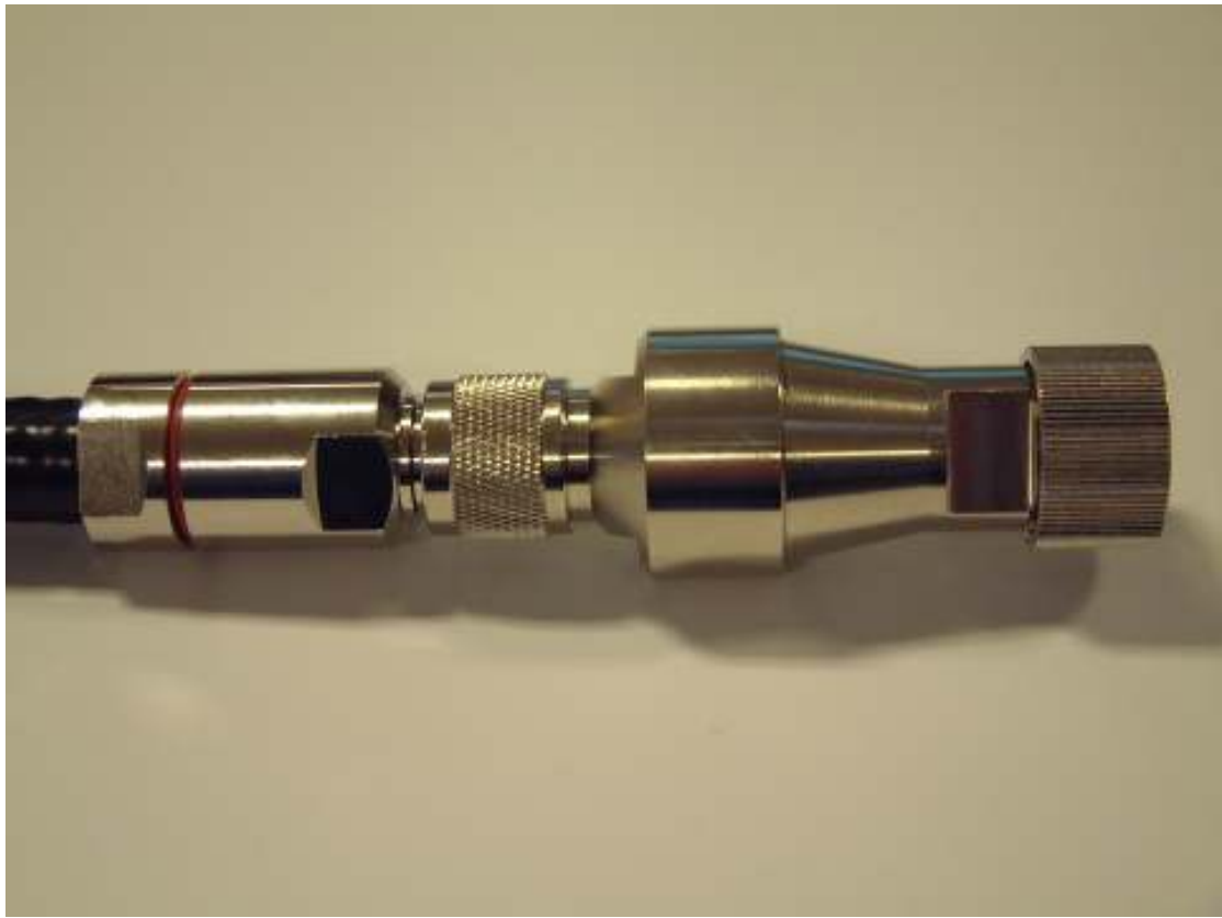
Final part with a terminator screwed onto the socket.
