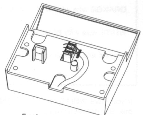
directly above the connector. Press down firmly – this will make the Connection.
