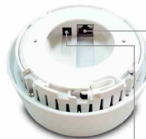
DC-inlet for Power Ethernet Port for RJ-45 cable
